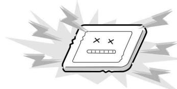
7. Do not expose the LCD module to direct sunlight or strong ultraviolet rays for an extended period of time.
