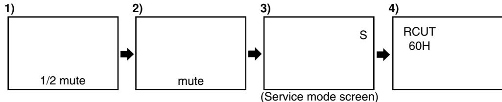
\* EXIT FROM SERVICE MODE-Turn off the "POWER" of the TV or remote control.
